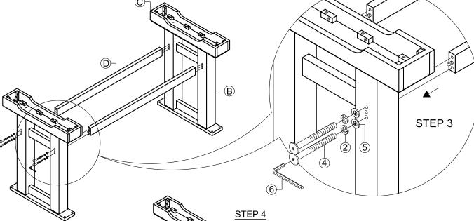
Turn the Table Top (I) upside down. Attach the Table Base Assembly in Step 3 to the Table Top (I) by inserting Large Flat Washer (3), Lock Washer (2), Short Bolt (1), and tighten by Allen Key (6). Put Screw Cover (E) into the holes of the Post as shown.
